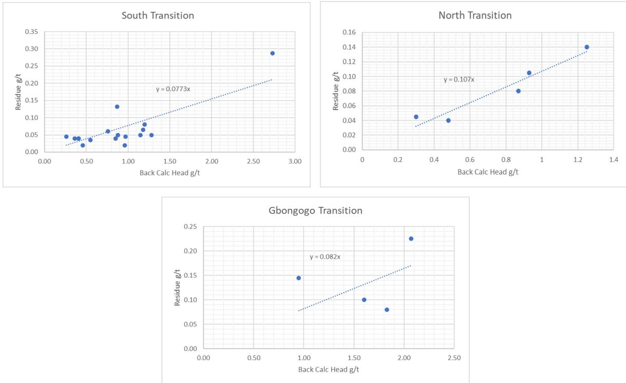
**Figure 13.4.3 Relationship Between Grade in Residues and Grade in Feed for Oxide Domains**
