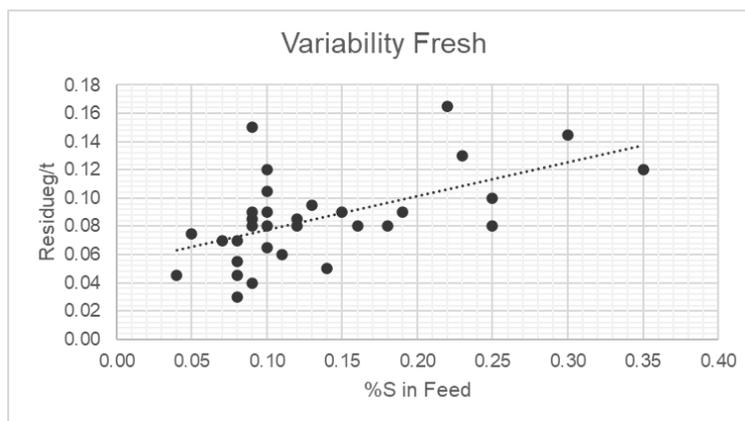
Figure 13.3.3 indicates that there is a linear relationship between feed sulphur and cyanide consumption. This was consistent across all samples tested.
