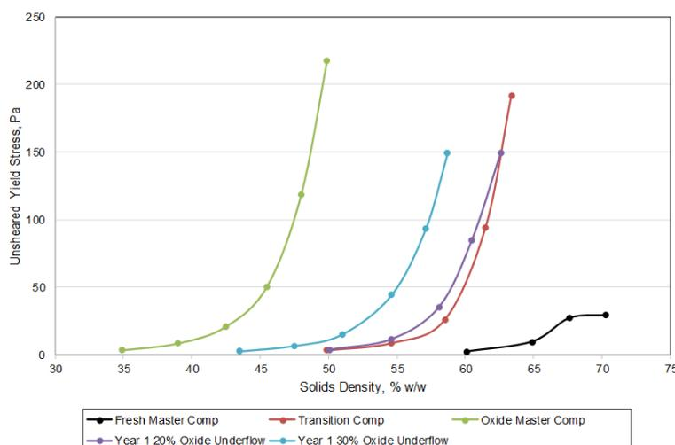
The thixotropic nature of the oxide mineralisation requires that the oxides are blended to <20% to maintain 50% solids feeding the leach circuit and avoid any adverse effects associated with carbon adsorption kinetics.
