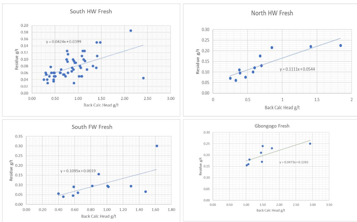
**Figure 13.4.2 Relationship Between Grade in Residues and Grade in Feed for Transition Domains**
