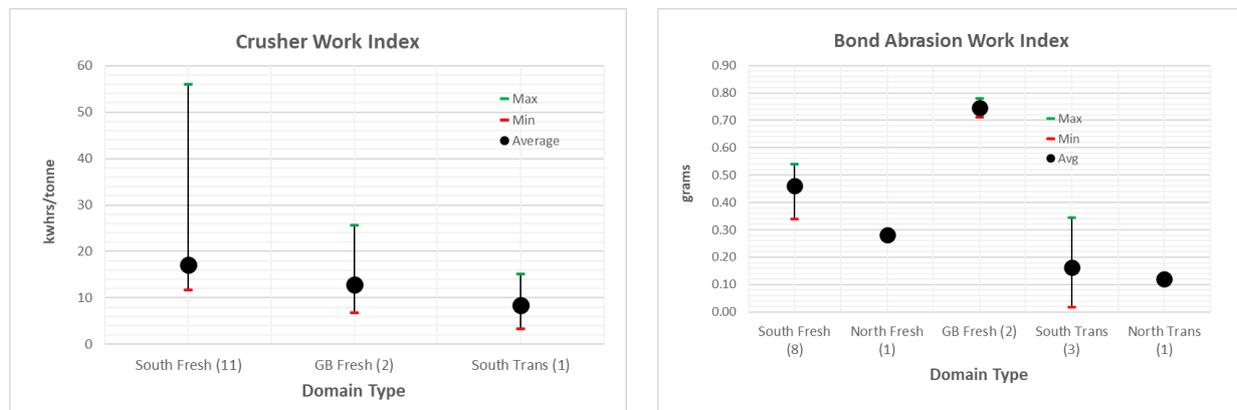
The fresh domains resistance to SAG milling was relatively consistently across all samples tested whereas the transition varies considerably, but is much softer. The oxide samples tested gave results that were all below JK Tech scale in terms of softness, this ore is extremely soft.
