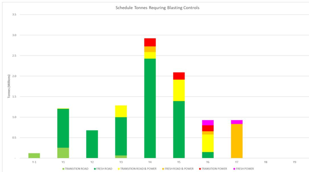
Controls will be put in place for blasting within a 500 m radius of powerlines to ensure that the blasting vibrations won't affect the powerlines. The blasting vibrations will be reduced to within acceptable levels by using programmable electronic detonators to control the output vibrations.
